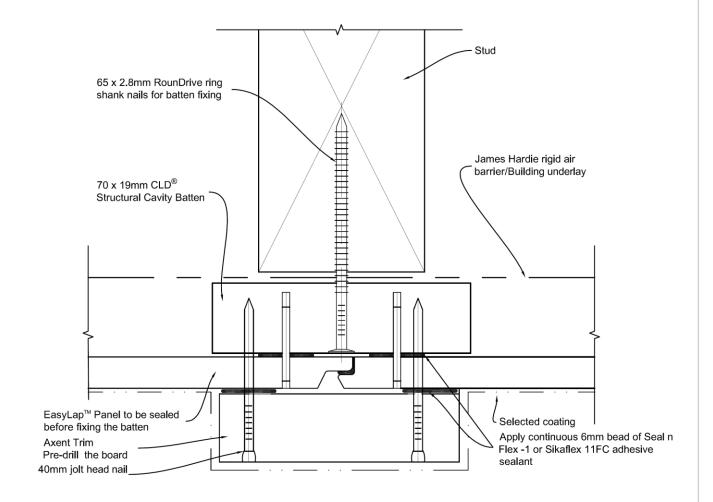
NOTE: Jolt head nails can be replaced with stainless steel brad nails.
